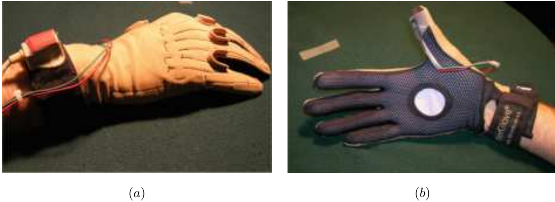
Figure 1: The devices used for the experiment, as worn by a subject: (a) the CyberGlove, with the Flock-of-Birds just above the subject’s wrist; (b) the Force Resistor Sensor attached to the subject’s thumb.
